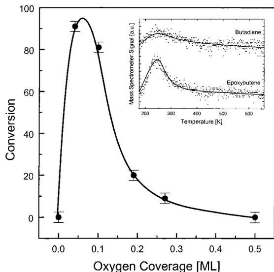
**Figure 2.** Conversion of butadiene to epoxybutene as a function of oxygen coverage over caesiated Cu{111},  $\theta_{\text{Cs}} \sim 0.07$  ML. Inset: Representative mass spectrum of butadiene and epoxybutene for  $\theta_{\text{O}} \sim 0.04$  ML.
