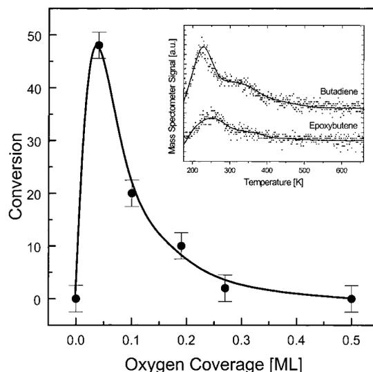
**Figure 1.** The conversion of butadiene to epoxybutene as a function of oxygen coverage over Cu{111}. Inset: Representative mass spectrum of butadiene and epoxybutene for  $\theta_{\text{O}} \sim 0.04$  ML.
