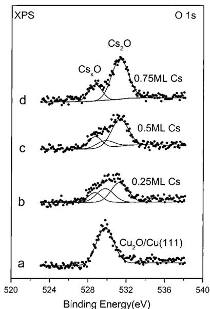
**Figure 3.** O 1s X-ray photoelectron spectra showing conversion of  $\text{Cu}_2\text{O}$  to Cu as a function of Cs dose: (a) no Cs; (b) 0.25 ML Cs; (c) 0.5 ML Cs; and (d) 0.75 ML Cs.
